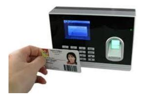
j) Biometric time clocks: These are a class of employee time clock that uses a person's biological attributes to identify them rather than using a cord or some other external device. Examples of this are the hand print clock which detects the overall attributes of a person's hand, fingerprint clock and retina scanning clock. Biometric item clocks help cut down on fraud such as buddy punching in which an individual clocks in and/or out on behalf of another person.
